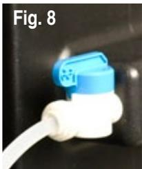
If you want to run the Dust Deputy® without the bag, you must shut the valve by turning the valve handle 90 degrees. The system must be air-tight to operate properly. Fig.8 shows valve in open position.
