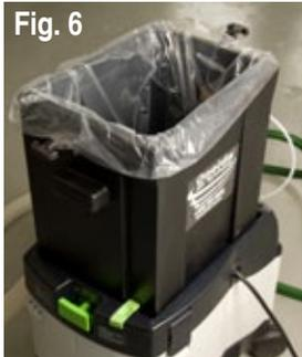
12. Place bag into box, tucking into corners and folding top of bag over top of box. (Fig. 6)
