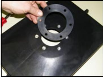
3. Put Gasket on box top making sure gasket holes line up with bolt holes in top.
