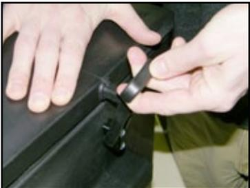
5. Pull up latch with grounding loops so hole in latch goes over the pin / boss on Dust Box top.
