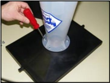
4. With a Phillips head screwdriver, attach the Cyclone with the (6) provided 1/4" x 20 x 3/4" bolts. Tighten in a star pattern as shown. Do NOT over tighten.
