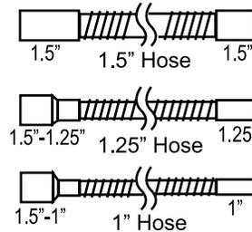
All hose is high quality, static dissipating, wire reinforced. All hoses have at least one 1.5" dia. cuff to attach to cyclone inlet.
