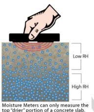
moisture is going to seek balance within the slab, as the surface airflow that wicks way migrating moisture is eliminated.
