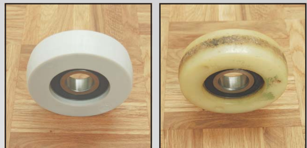
Pic. 9 Two sets of wheels (new + old) are helpful when sanding old dirty floors.
