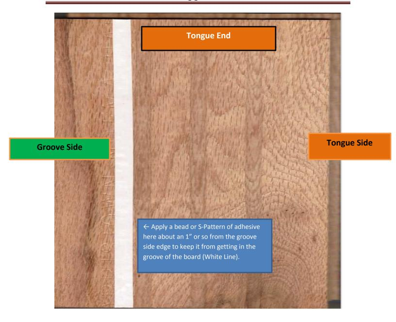
Relative Humidity variations result in either shrink or swell to occur across the width of the board, the wider the plank, the greater the percentage of movement.
